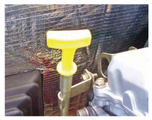
Figure 4.3 — Oil Dipstick and Fill, 12, 14, 16, 17 & 20kW
