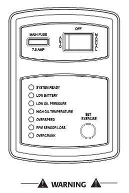
With the switch set to AUTO, the engine may crank and start at any time without warning. Such automatic starting occurs when utility power source voltage droops below a preset level or during the normal exercise cycle. To prevent possible injury that might be caused by such sudden starts, always set the switch to OFF and remove the fuses before working on or around the generator or transfer switch. Then, place a "DO NOT OPERATE" tag on the generator panel and on the transfer switch.
